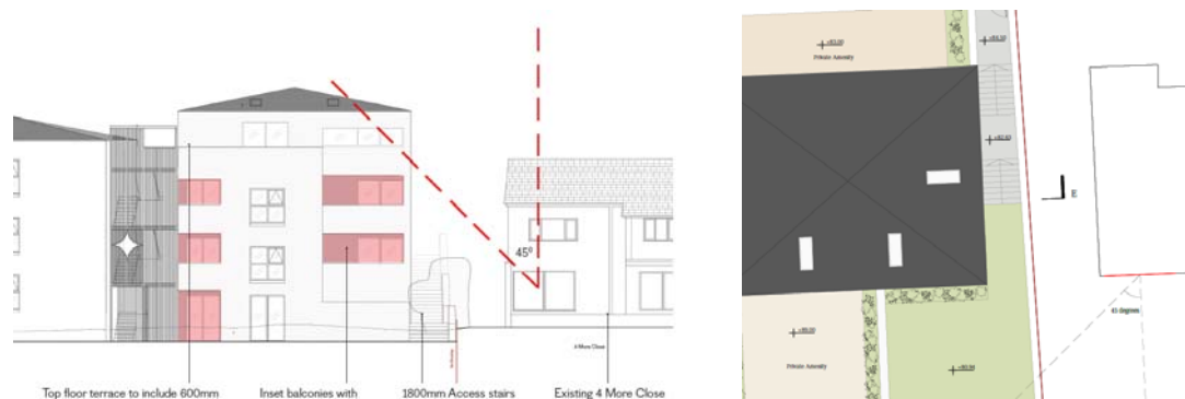
Fig.8: The 45° line from adjoining existing rear windows at No.4.
